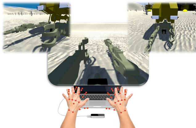
Fig. 4. ROV for offshore underwater maintenance controlled by LM.
